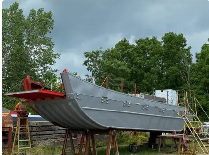
1995 30' x 10'3 Steel Landing Craft - 6 cyl Diesel w/ Azipod
